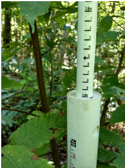
Figure 1. (Left) Tall seedlings were measured with a telescopic measuring rod like this one at EPRR. (Right) Hemispherical photography is used to measure canopy openness at a small gap site at Barker Pounds.
